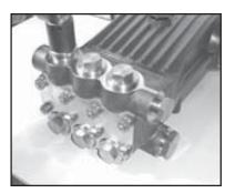
15. Replace plug with o-ring (48, & 48A) and tighten to 160 ft.-lbs.
